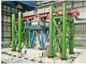
▲ A next generation damage-free RC bridge column placed on top of the 20m x 15m shaking table
