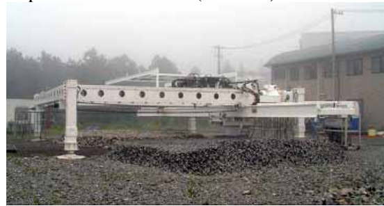
Photo.3 Underwater Grading Robot
