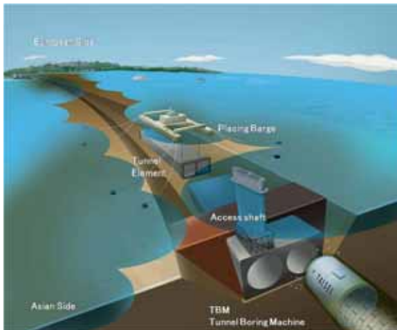
Fig.4 Bird's-Eye View of the Immersed Tunnel
