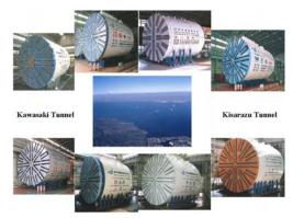
Fig.1-2 Large Bore in Trans-Tokyo Bay Highway
