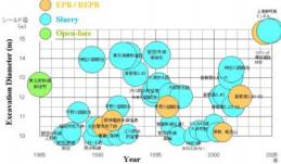
Figure 1-1 Large circular shield with excavation diameter of 10m or over (continue page2)
