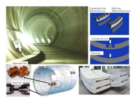
Figure 4 RC Lining Segment with Rigidity Controllable One-Pass Joints
