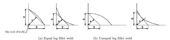
Fig.C11.5.4 Theoretical throat thickness of fillet weld
