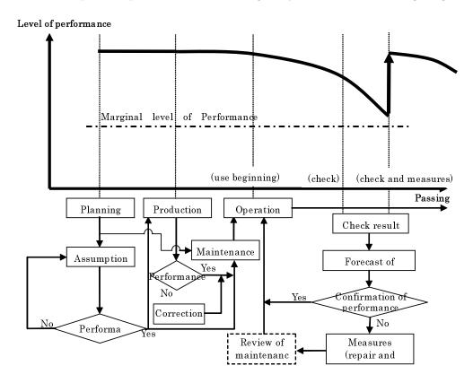
Fig.C1.2.1 Performance of structure during its life cycle
