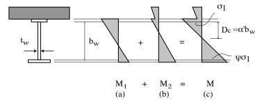
Fig.C15.2.3 Superposition of stress in unshored composite girder
