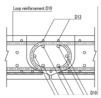
Fig.C14.6.1 Loop joint
