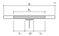
Fig.C15.7.1 Definitions of effective width  $B_e$  and total width B
