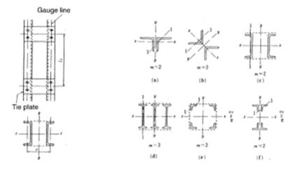
Fig.C12.2.5 Built-up compression members (tie plates)
