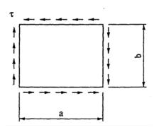
Fig.C5.3.8 Distance between fixed edges of plate
