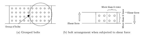
Fig.C11.7.2 Minimum number of high-strength bolts
