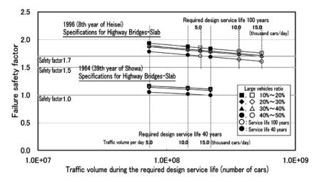
$Fig. C14.4.2\ Typical\ evaluation\ of\ fatigue\ durability\ by\ safety\ factor\ [Kawabata\ et\ al.\ 2004b]$
