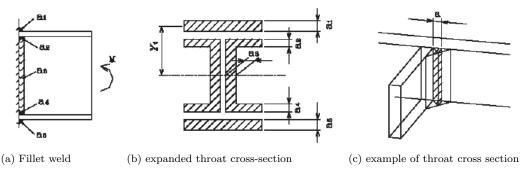
Fig.C11.5.1 Fillet weld connection subjected to bending moment
