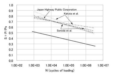
Fig.C14.4.1 Typical S-N curve (Osaka University) [JSCE, 2004b]
