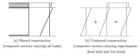
Fig.C15.1.1 Stress in composite girders
