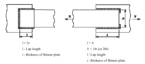
Fig.C11.5.11 Lap joint by fillet welding
