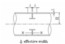
Fig.C10.6.4 Effective width of steel tube
