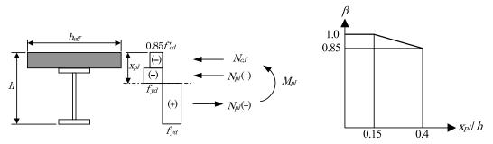
Fig.C15.2.5 Reduction factor  $\beta$  (positive: tension)
