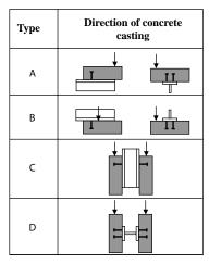
Fig.C15.4.2 Classification of headed studs depending on concreting irection
