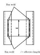
Fig.C11.5.8 Effective length of weld
