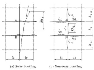
Fig.C12.2.12 Buckling of multi-storey framework
