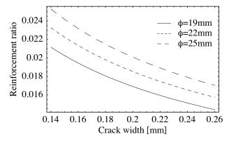
Fig.C15.6.1 Relationship between reinforcement ratio and crack width in initial crack state (concrete tensile strength=  $2.5 \mathrm{N/mm}^2$ ,  $\epsilon_{csd} = -150 \mu$ )
