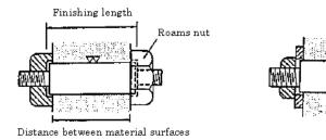
Fig.C11.9.1 Pin and nut
