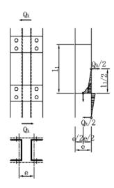
Fig.C12.2.11  $Q_k$  of a girder combination member
