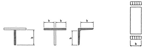
Fig.C5.3.6 Width of cantilever part of plate supported at one edge
