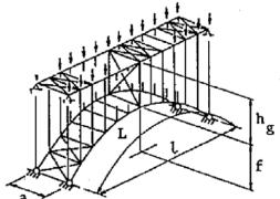
Fig.C12.2.14 Half-through type arch
