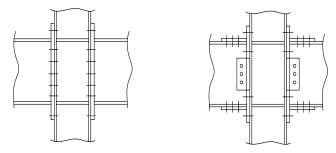
Fig.C11.6.5 Examples of tension-type connections
