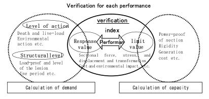
Fig.C2.2.1 Framework of performance verification
