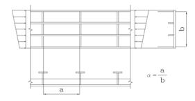
Fig.C10.4.4 Longitudinal and transversal dimension ratio of stiffener
