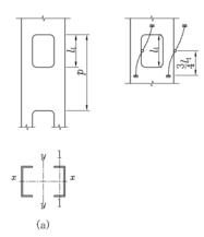
Fig.C12.2.9 Cover plates with holes
