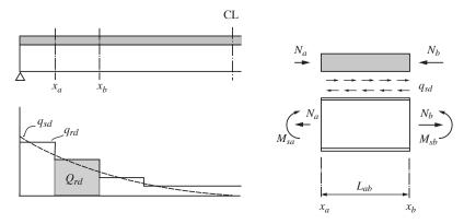
Fig.C15.4.1 Horizontal design shear force and design strength
