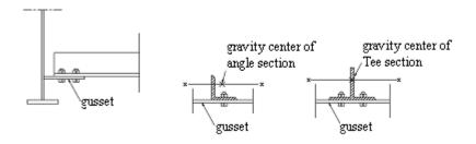
Fig.C10.4.6 Compression member comprising angle or T section
