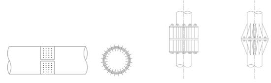
Fig.C10.6.6 Example of 4-way splitting of a restrainer plate
