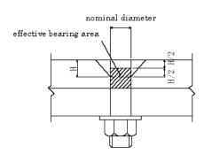
Fig.C11.6.4 Effective bearing area of flat-head bolt
