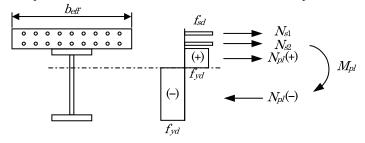
(b) When plastic neutral axis is within the web receiving negative bending Fig.C15.2.4 Examples of plastic stress distributions for a composite girder in positive or negative bending moment (positive: tension)
