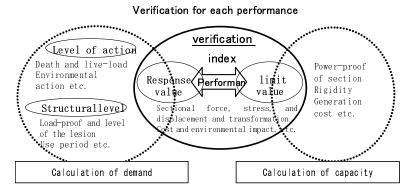
Fig.C1.4.1 Framework of performance verification
