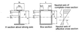
Fig.C5.3.1 Effective Sections of Beams
