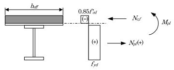
(a) When plastic neutral axis is within the concrete deck in positive bending
