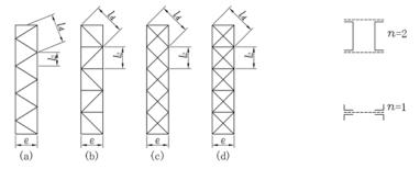
Fig.C12.2.7 Built-up compression members formed by lacing bars
