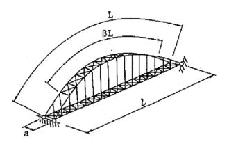
Fig.C12.2.13 Through type arch
