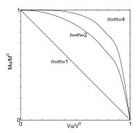
Fig.C15.2.6 Shear-moment interaction diagram
