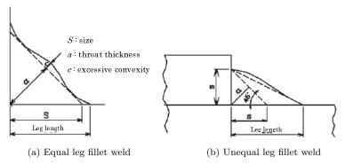
Fig.C11.5.9 Fillet weld size
