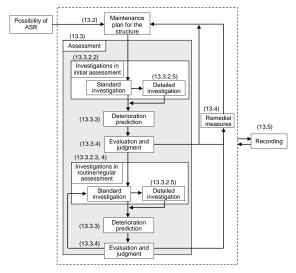
Fig. C13.1.2 Standard maintenance procedure against ASR
