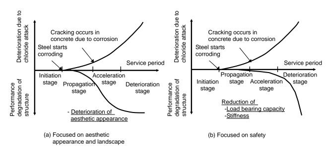
Fig. C10.1.1 Progress of deterioration progress due to chloride attack
