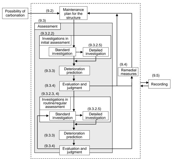
Fig. C9.1.2 Standard maintenance procedure against carbonation
