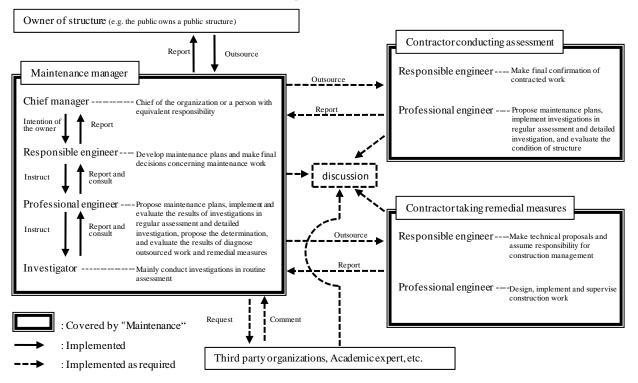
Fig. C1.2.1 Examples of a system for structure maintenance and roles of engineers
