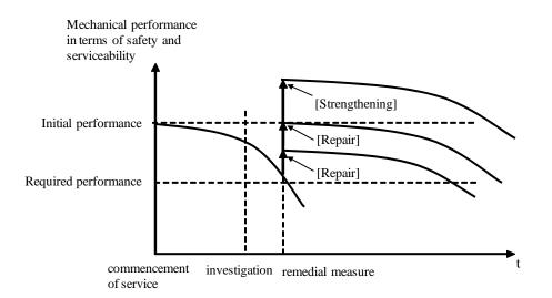
Fig. C1.3.2 Definitions of repair and strengthening
