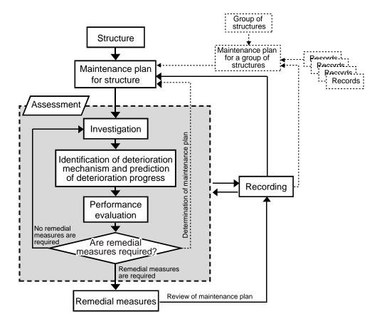
Fig. C3.1.1 Procedure for maintaining a structure
