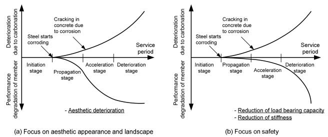
Fig. C9.1.1 Conceptual view of deterioration progress due to carbonation
