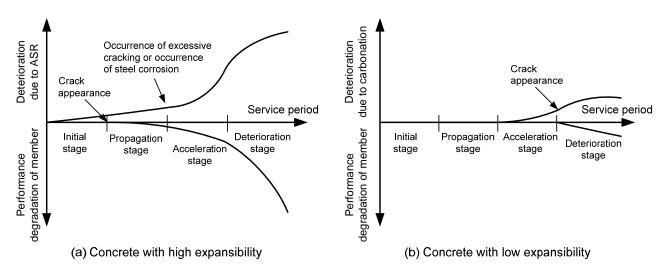
Fig. C13.1.1 Conceptual view of deterioration progress due to ASR
