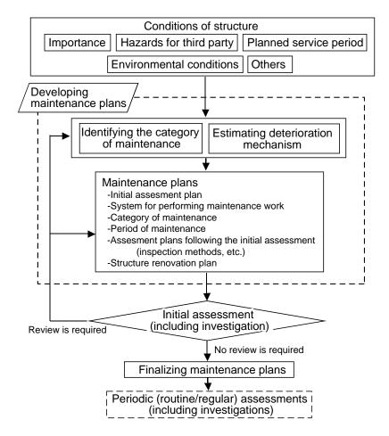
Fig. C3.2.1 Procedure for developing maintenance plans
