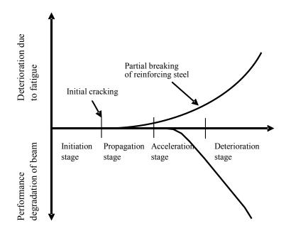
Fig. C15.1.1 Conceptual view of deterioration progress due to fatigue-induced of beam
