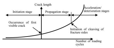
Fig. C15.3.1 Model of fatigue crack propagation in reinforcing steel
