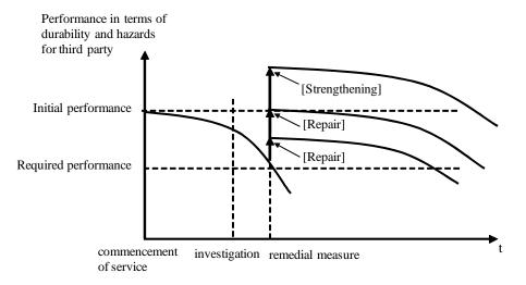
Fig. C1.3.2 Definitions of repair and strengthening
