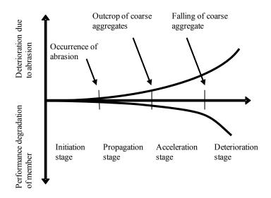
Fig. C16.1.1 Conceptual view of deterioration progress due to abrasion
