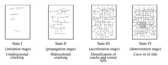
Fig. C14.3.1 Progress of cracking at underside of reinforced concrete slab
