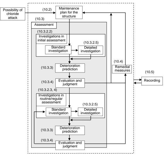
Fig. C10.1.2 Standard maintenance procedure against chloride attack
