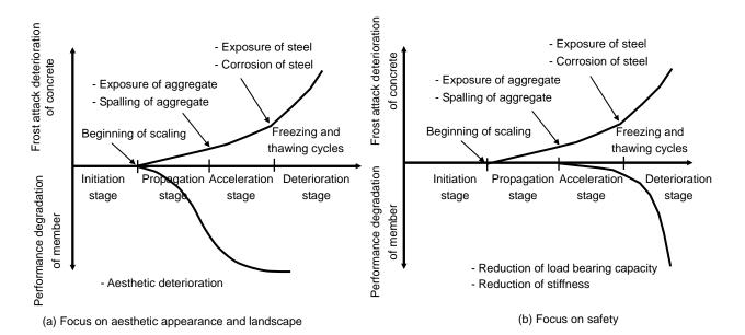
Fig. C11.1.1 Conceptual view of deterioration progress due to frost attack
