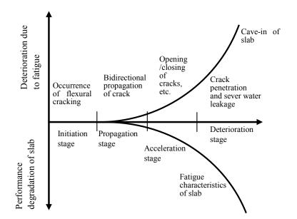
Fig. C14.1.1 Conceptual view of deterioration progress due to fatigue of concrete slab
