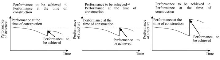
(i)Restoration of performance to a level midway between the time of construction and present, or maintenance of present level of performance
