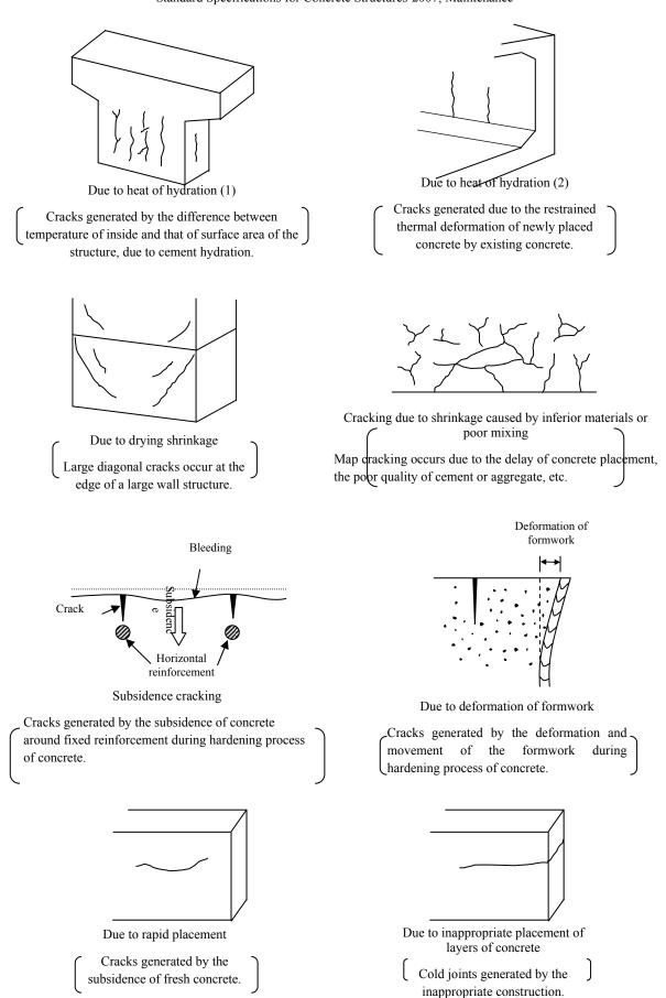
Fig. C5.2.1 Examples of initial cracks occurring during construction
