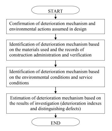
Fig. C5.1.1 Basic sequence for identification of deterioration mechanism
