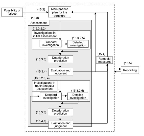
Fig. C15.1.2 Standard maintenance procedure of beam under fatigue stress
