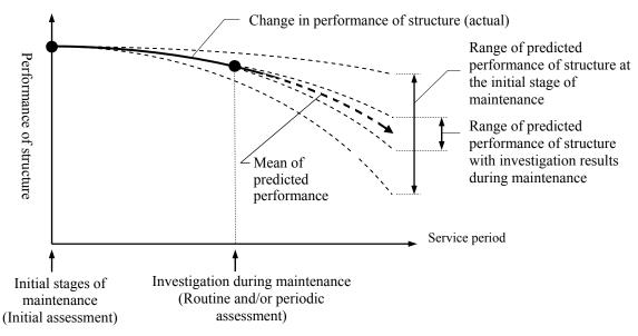
Fig. C5.3.1 Accuracy of deterioration prediction
