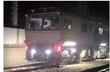
Mechanical vehicle correcting track irregularity (Multiple tie tamper)
