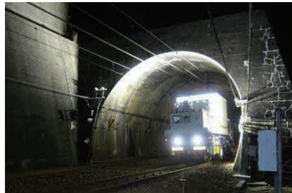
Tunnel inspection vehicle using laser light (vehicle taking images of the surface of tunnel linings)
