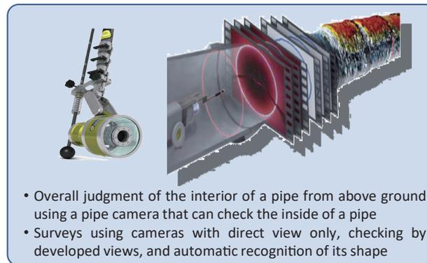
Fig. Pipeline inspection system using wide-angle camera
