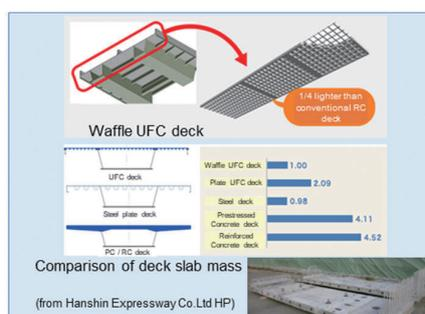
Deck slab replacement method using ultra high-strength fiber-reinforced concrete (UFC) deck slabs, which are lighter than conventional RC or PC deck slabs and have greater durability
