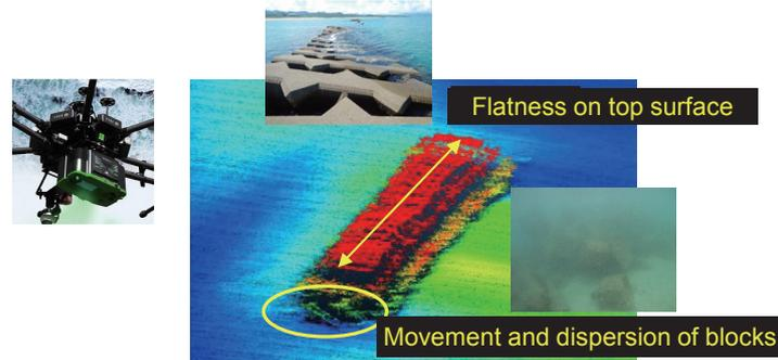
Fig. Example of shape measurement (detached breakwater)
