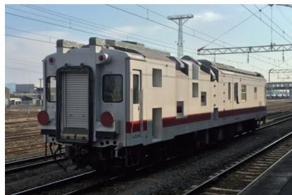
Vehicle checking for obstacles around tracks using laser light (structure gauge measurement vehicle)
