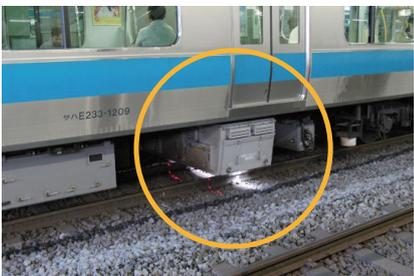
Monitoring at high frequency using operating trains
