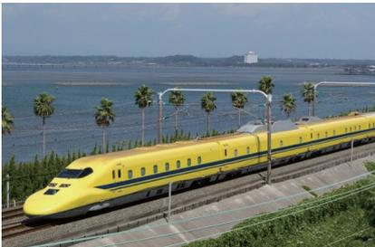
Multiple inspection train for inspection of Shinkansen tracks and electrical equipment (Doctor Yellow)
