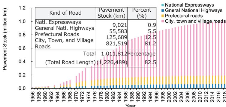
Fig. Total length of paved road including pavements for light traffic (Source: the Annual Report of Road Statistics 2020)
