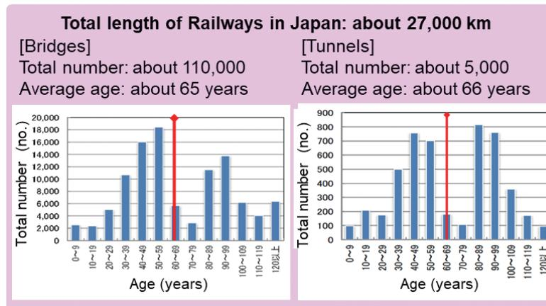
Fig. Age distribution of railway bridges and tunnels
