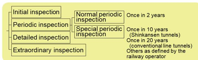
Fig. Categories of railway structure inspections
