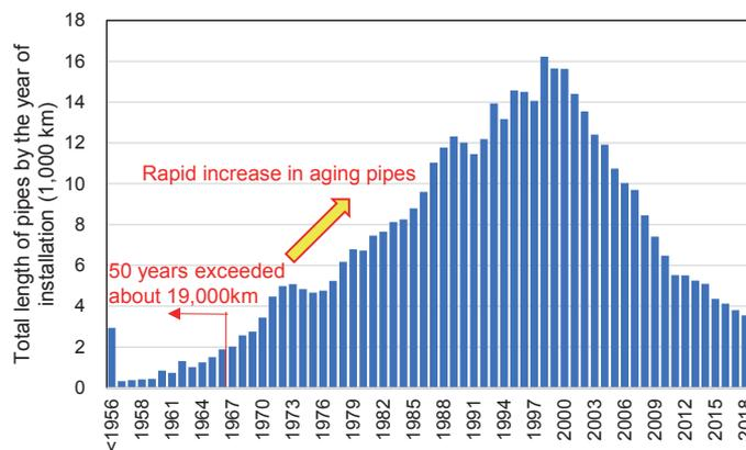
Fig. Total length of pipes as of end FY 2018 (prepared from Ministry of Land, Infrastructure, Transport and tourism document)
