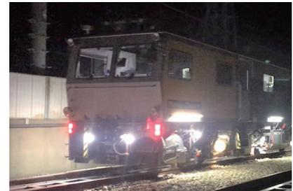
Mechanical vehicle correcting track irregularity (Multiple tie tamper)
