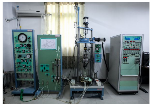
Photo 1 Soil testing apparatus in Shanghai Jiao Tong University (small-strain triaxial, hollow cylinder)
