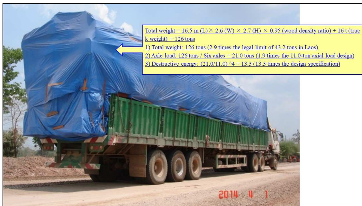
Overloaded trailer transporting blocks of wood (broke down in the center of the road due to the vehicle being too heavy)
