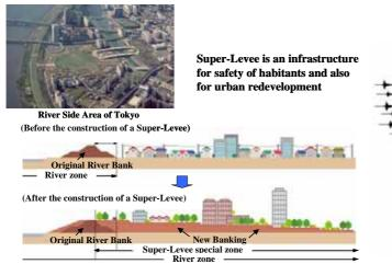
Figure 17 Construction of the Super-Levee in Low Land Area of Tokyo against Future Earthquake
