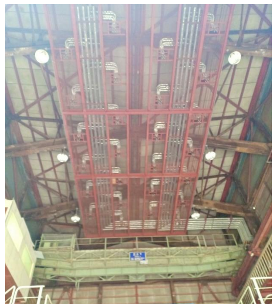
Figure 13.0 Large – Scale Rainfall Simulator
