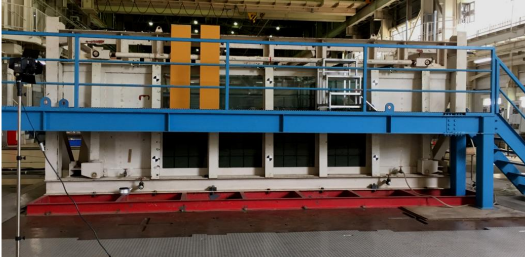
Photo 5, Three-Dimensional Shaking Table
